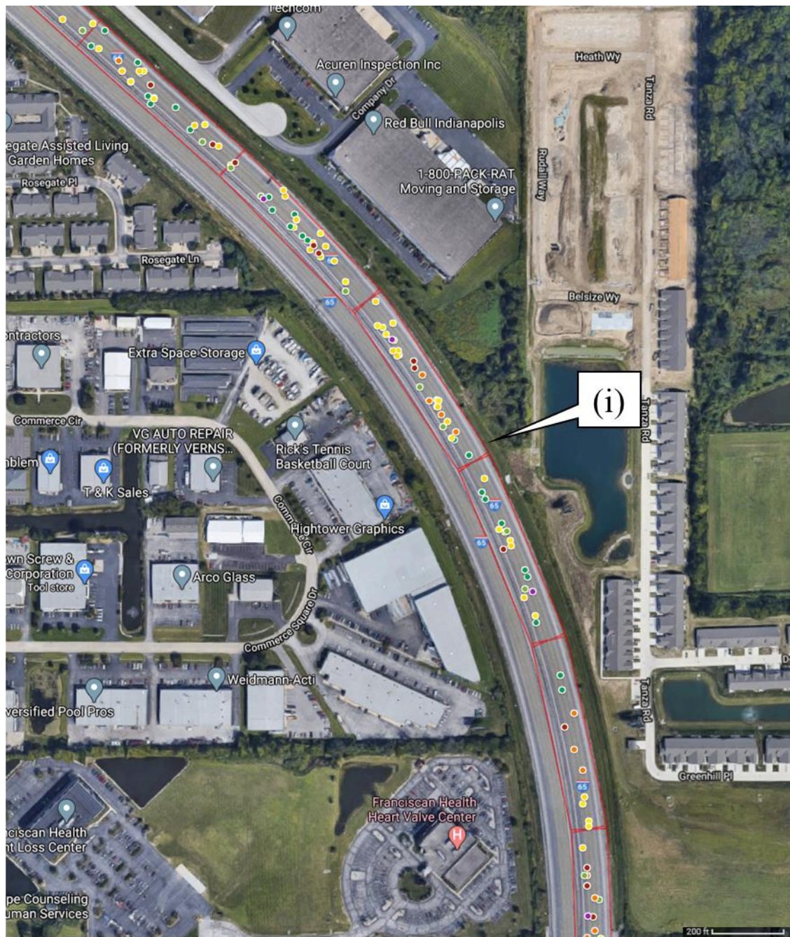
Figure 22. Geofenced polygons showing hard-braking events colorized by initial speed in miles per hour on I-65 in the northbound direction of travel in the vicinity of mile marker 102
