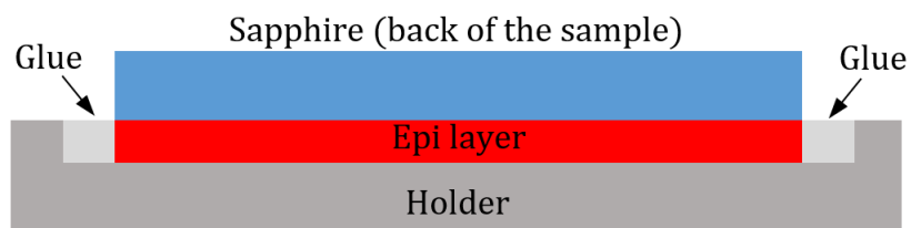
Figure A.1. Cross-section view of mounting plan-view sample onto PIPS holder before milling.
