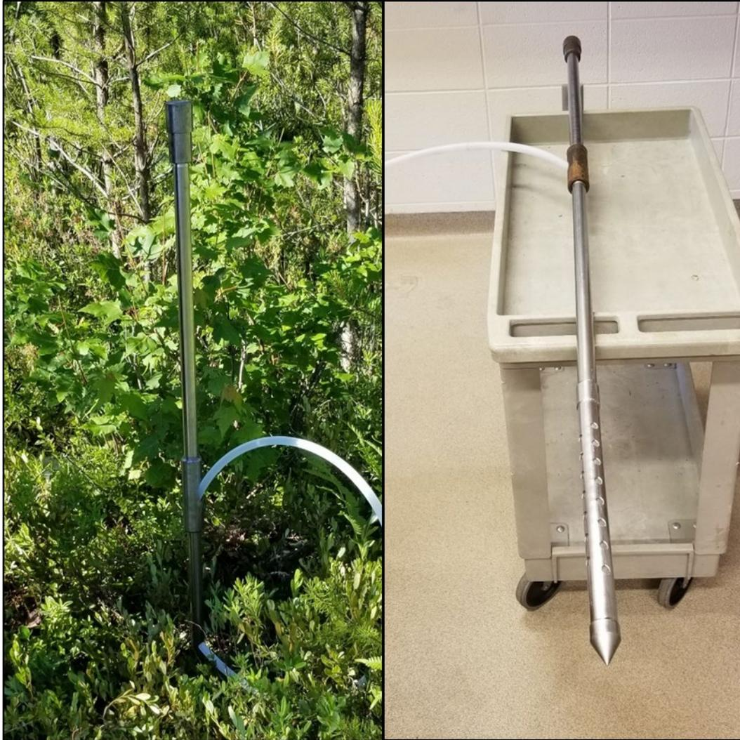
Figure 4. Drive point well apparatus used to pump ground water to the surface at each sampling point. Wells were driven to ~1 meter depth with a slide hammer. Piezometers (portion shown with openings above the tip), extension tubes, and white tubing were soaked in 50% bleach before each use.
