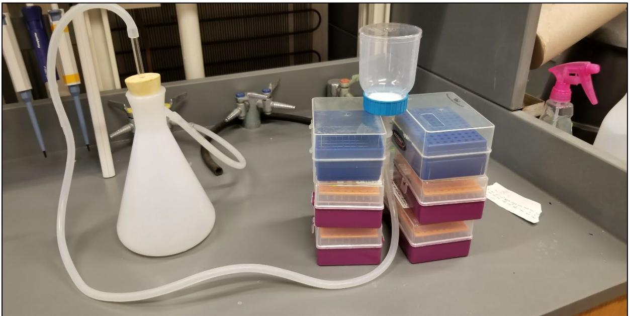
Figure 5. Ground water filtering set up, consisting of the Nalgene filter unit connected to tubing that flows into a collection flask for flow through. The apparatus is connected to in house vacuum unit.
