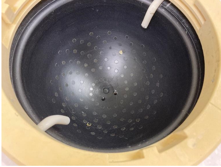
Figure 10: In-house detector (NEXUS128) with sub- 2\pi angular coverage. The small circles are individual transducers.
