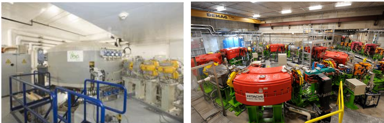
Figure 2: Cyclotron (left) and synchrotron (right). (Image source (left): OncoLink, Proton Therapy: Behind the Scenes . Image source (right): MedGadget, Hitachi Proton Beam Therapy Coming to Mayo Clinic .).
