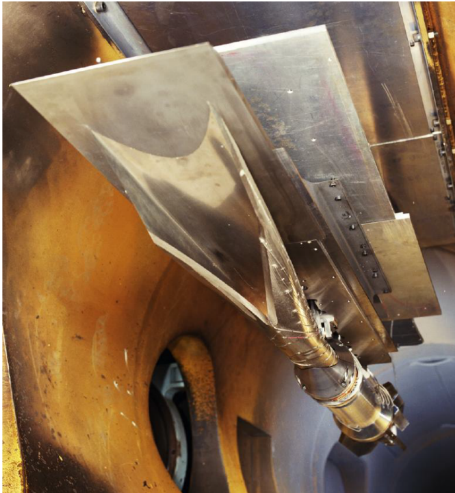
Figure 2.6. Isometric view of the shape-transitioned REST intake undergoing testing at NASA Langley [82]. Reprinted by permission of the American Institute of Aeronautics and Astronautics, Inc.
