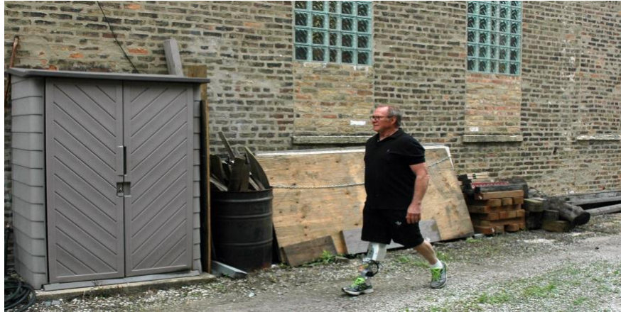
Note: Robotic powered prosthetic leg using electromyographic (EMG) signals. (Advanced Control Systems for Powered Prosthetic Legs, 2016)
