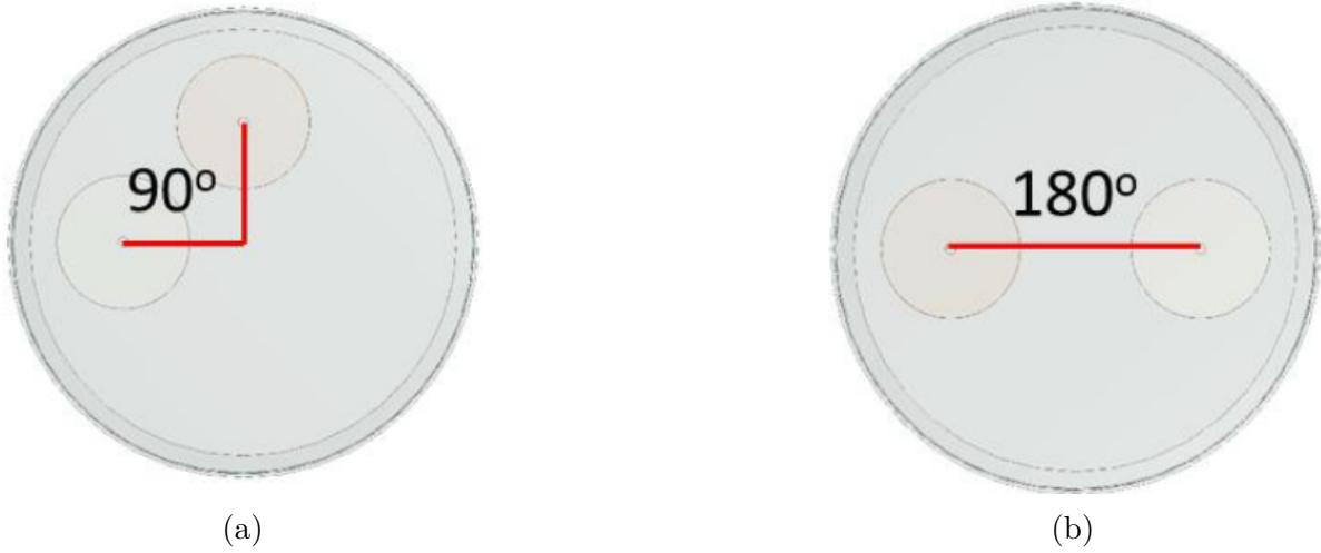
Figure 2.2. Schematic diagram of different plug separation angles: (a) 90^\circ ; (b) 180^\circ .
