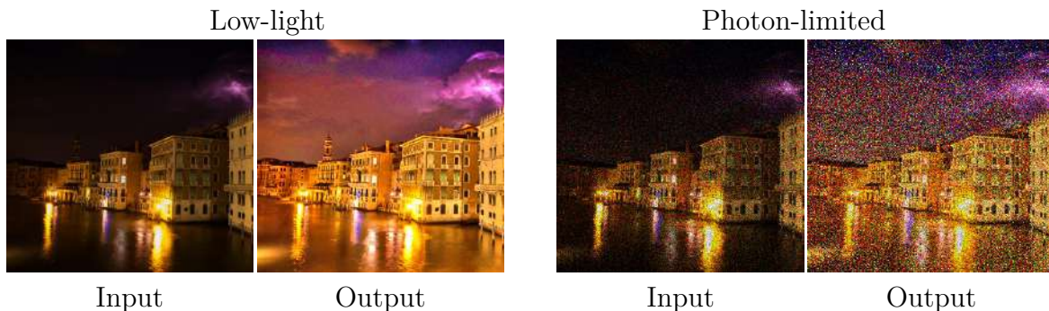
Figure 1.20. Low light image enhancement. We can notice that the low light image enhancement using [19] works well when noise is absent, even though the image appears dark. However, when the scene is corrupted by heavy shot noise, which is what we are interested in this dissertation, the method does not perform that well.
