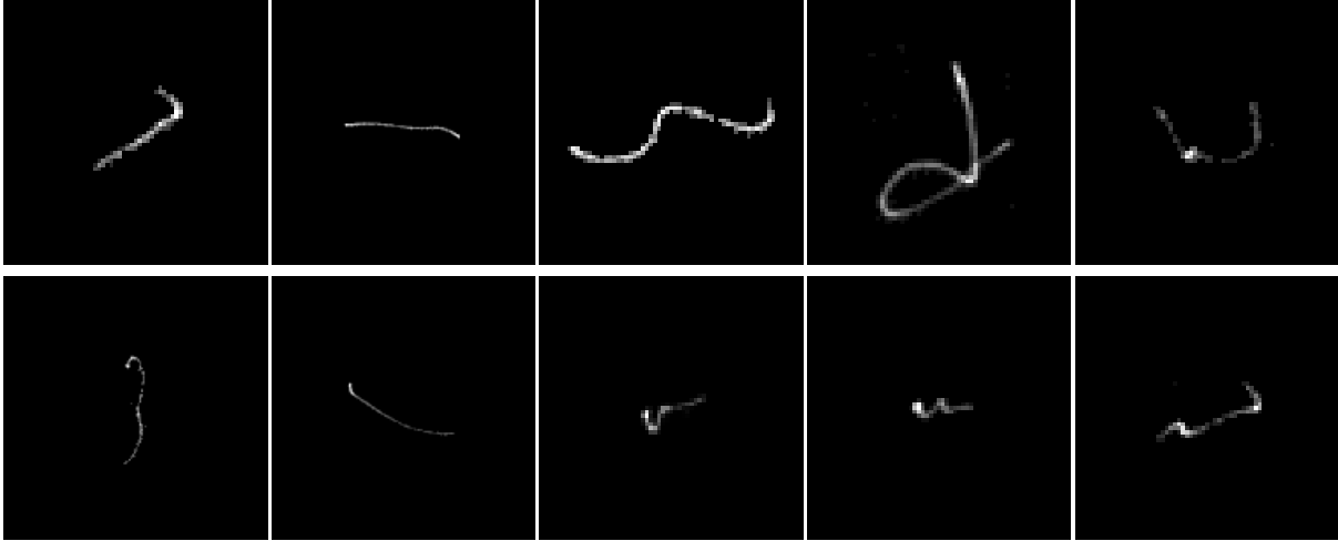
Figure 6.11. Real kernels generated by our optical experiment setup.
