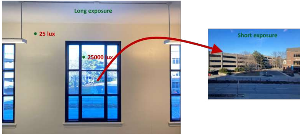
Figure 1.17. High dynamic range. We can see that the camera is capable of capturing all the light levels in this scene, however it is not able to capture them in a single image.
