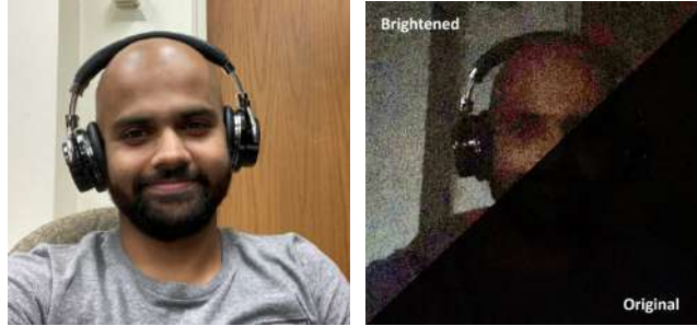
Figure 1.12. Imaging at low light. The same scene is captured with and without external illumination using an iPhone. The image on the right is brightened for better visualization. We can clearly notice the poor signal to noise ratio in the right image.
