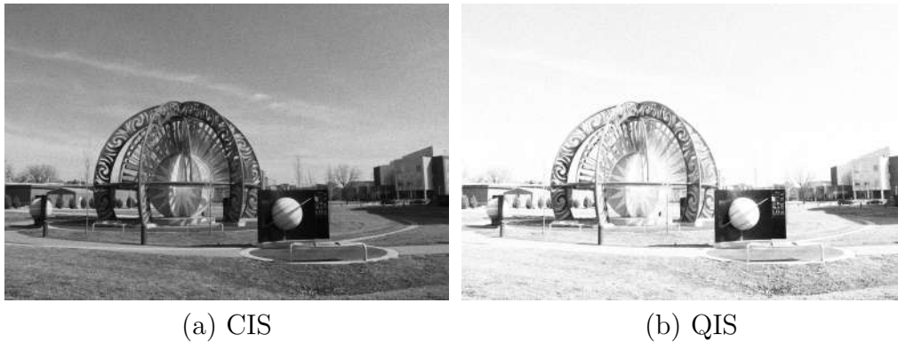
Figure 8.2. Dynamic range of quanta image sensors. The lower bit depth of QIS severely affects the full-well capacity and, in turn, the dynamic range of the image sensor. The QIS image is heavily washed out even at an average of 10 photons per pixel (ppp). However, all hope is not lost. Please keep reading to see how we can use QIS to get a dynamic range even more significant than a CIS.
