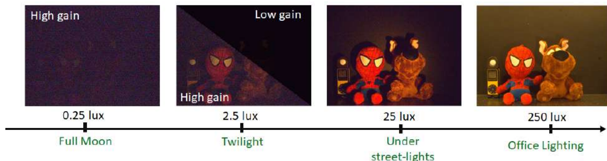
Figure 1.11. Imaging low-light scenes. All the images here are captured using Thorlabs CS165CU camera with integration time of 30ms. As the light level goes down, we can notice that the camera struggles to capture a good enough image.
