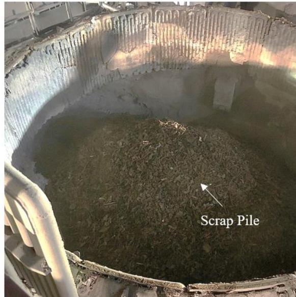
Figure 3.45. NLMK EAF with scrap charged;
