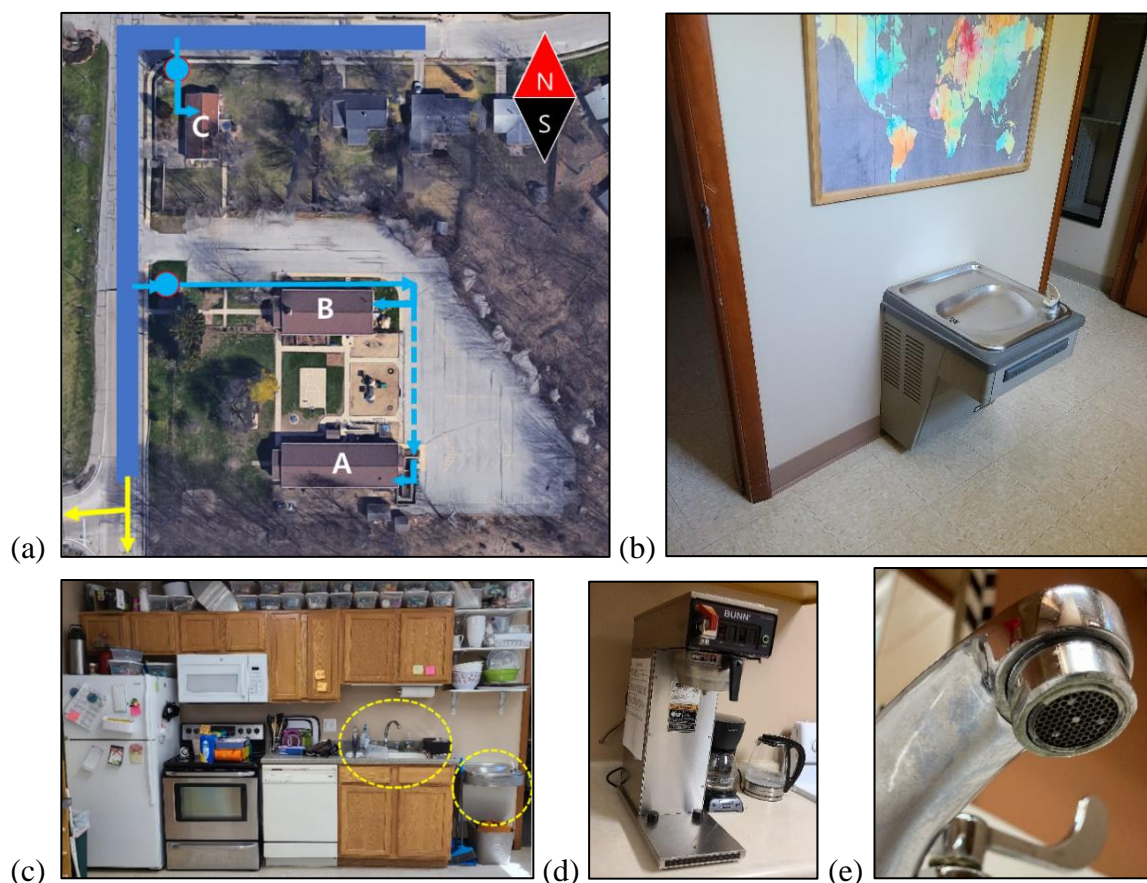
Figure 3-1. (a) Site property with building A, B and C with estimated location of public water supply pipe (blue), two water meters (sky blue circle) and service line to each building (sky blue) and where splits to deliver to building A (dotted sky blue), (b) Elkay drinking water fountains installed for kids' height, (c) All classrooms had their own sinks, drinking water fountain, and appliances, (d) Coffee maker connected to the plumbing in building A, and (e) Particulates on the aerator before removal.
