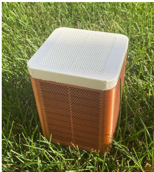
Figure 6. An example of the set-up used to attract blow flies (aerated vessel containing rotting meat).
