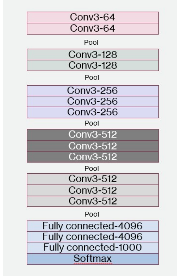
Figure 3.2. Model structure for VGG-16
