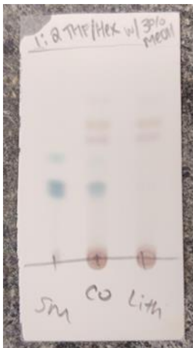
Figure C.13. TLC plate of the literature synthesis \text{Ru}_2(\text{amtfmp})_4\text{Cl}_2 material (left lane, abbreviated as 'SM'), a co-spot of the literature material and the crude lithiation product (center lane, abbreviated as 'Co'), and the crude aryl lithiation product (right lane, abbreviated as 'Lith')
