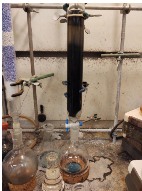
Figure C.12. Column purification of \text{Ru}_2(\text{amtftp})_4\text{Cl}_2 . The excess ligand was removed by running \text{CHCl}_3 , the product ( \text{Ru}_2(\text{amtftp})_4\text{Cl}_2 ) removed with \text{CHCl}_3 with 5% \text{MeOH} (v/v)
