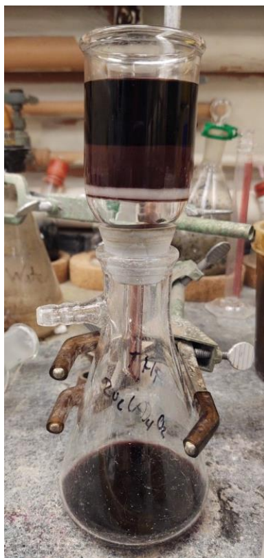
Figure C.11. Filtration of crude \text{Ru}_4(\text{amtftp})_4\text{Cl}_2 through Celite to remove excess \text{LiCl} . Solution was a dark red-purple
