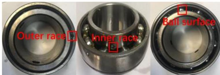
Figure 2-5 The location and shape of the bearing defect
