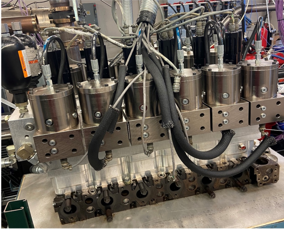
Figure 4.1. VVA standalone system in test cell.
