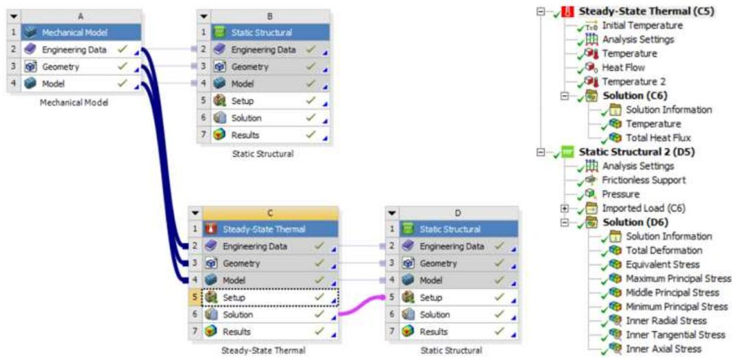
Figure 4.6: ANSYS Workbench setup for thermo-elastic stress verification.
