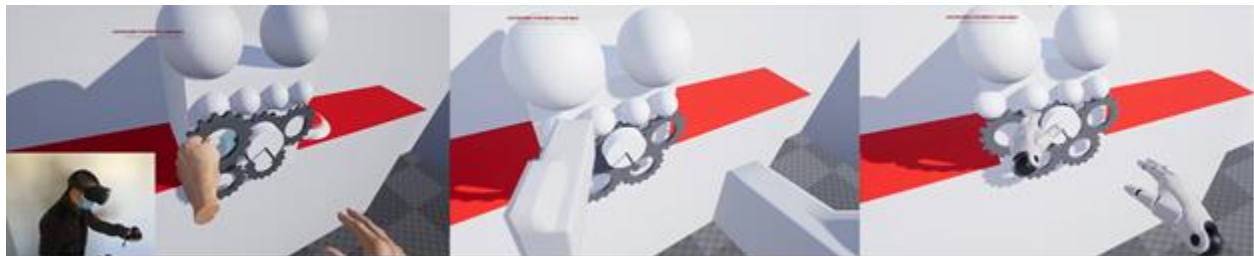
Figure 43. A participant assembling a gear part in the virtual environment with all three hand models (from the left: realistic, abstract, mannequin).
