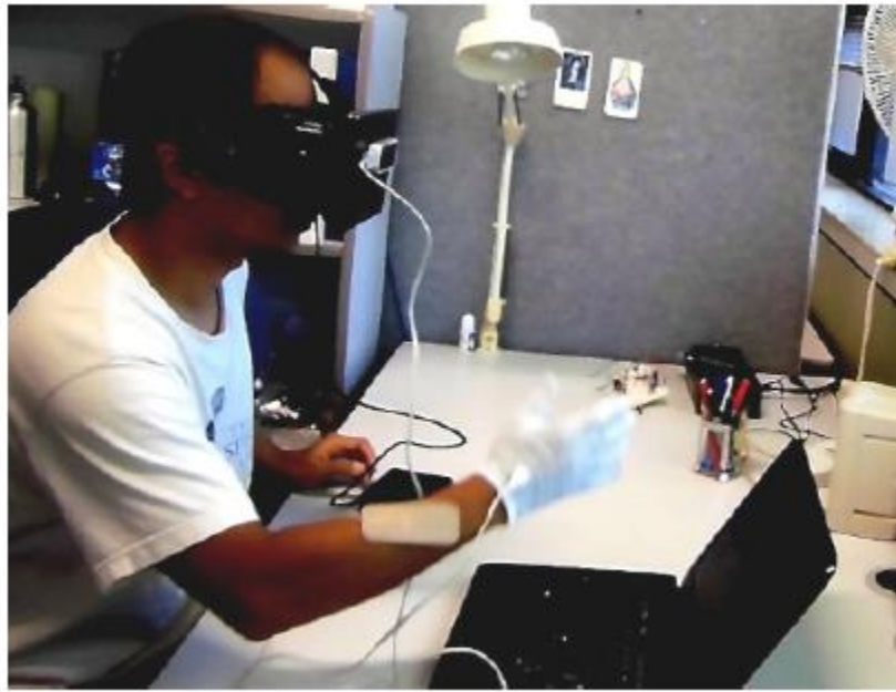
Figure 15. User using the electro-tactile feedback system with Oculus Rift, Leap Motion hand tracker and the haptic feedback device [86].
