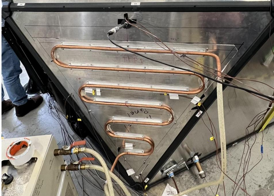
Figure 9: Triangular Thermal Transfer Panel
