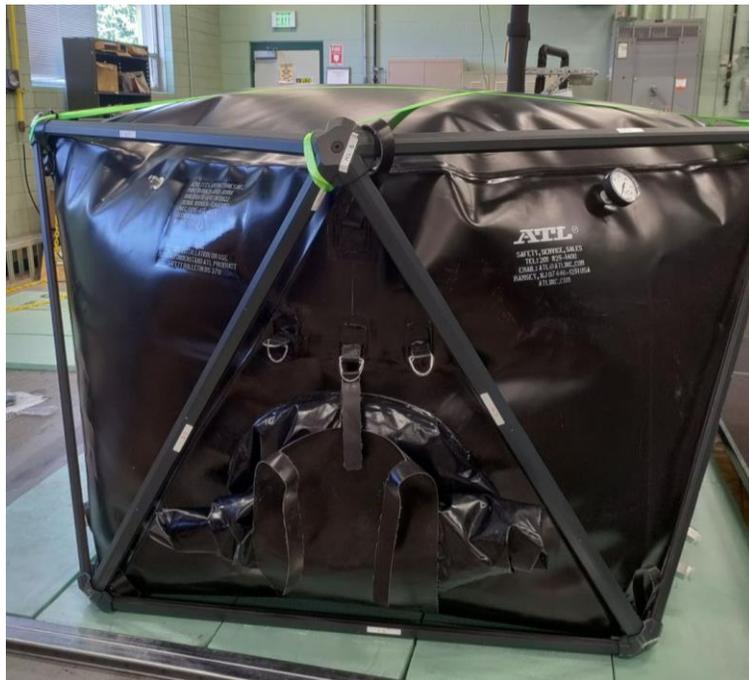
Figure 8: Habitat Prototype Consisting of Geodesic Dome and Inflatable Bladder
