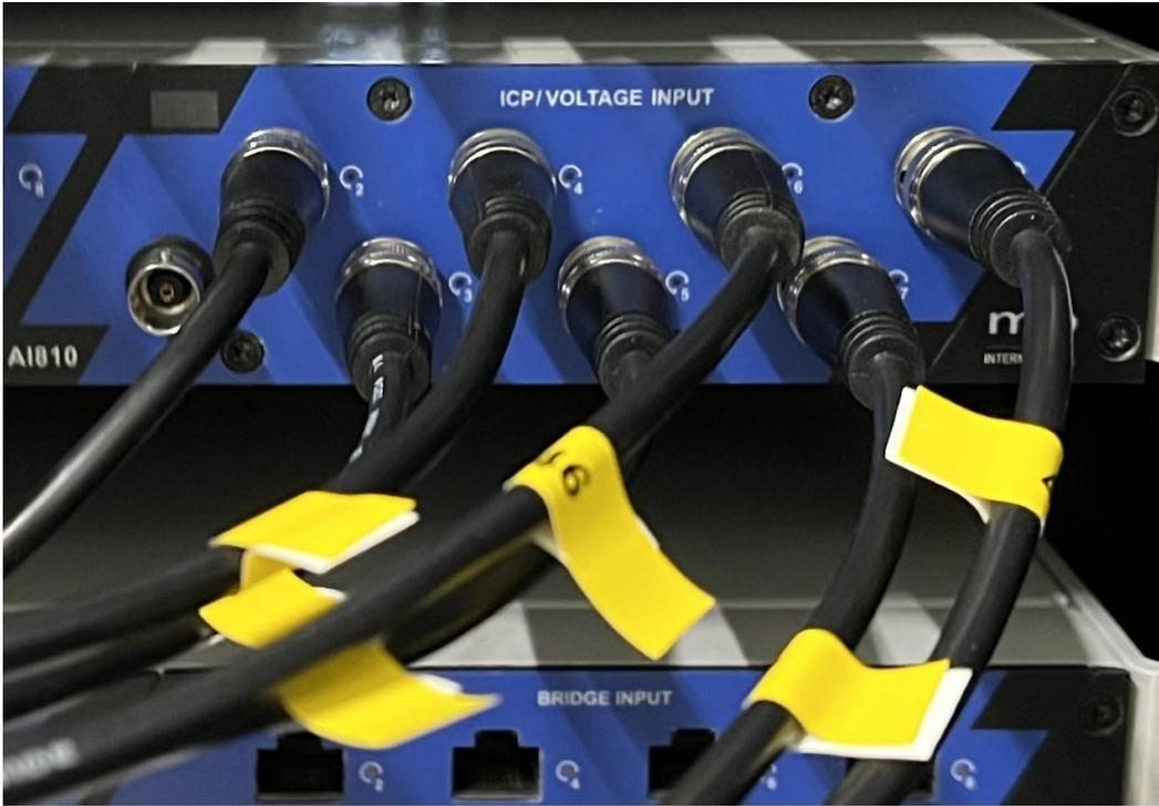
Figure 13: Sensor Inputs to Voltage I/O Module
