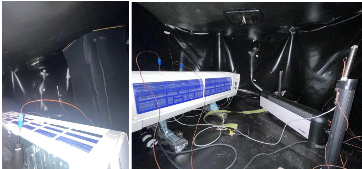
Figure 46-The box which contains four lamps (left) and the heater to the right of the unit of the mini-split (right)
