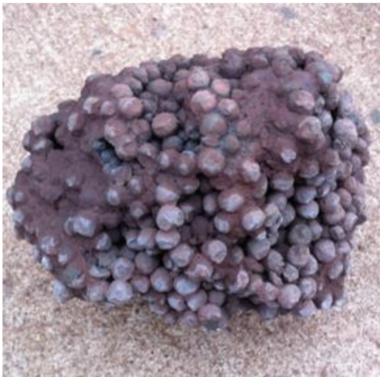
Figure 60. Example of pellets frozen together from being exposed to winter conditions in an ore field
